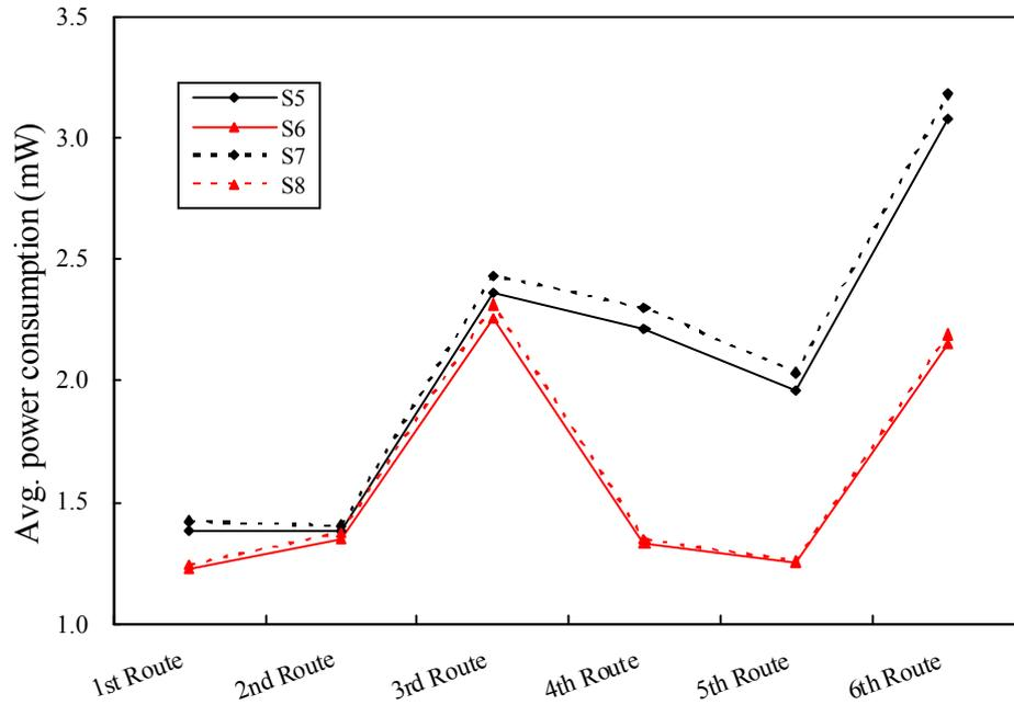
Figure 5-9: Average power consumption by using ARQ scheme.
