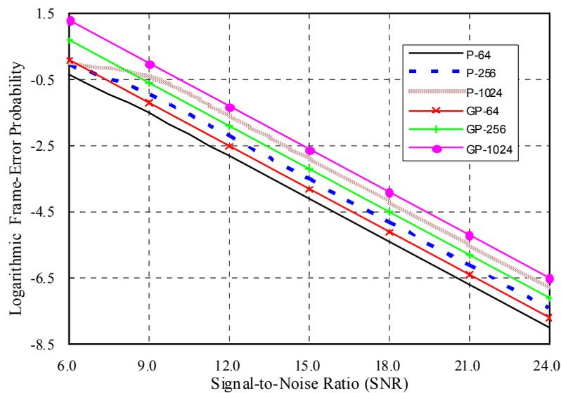
(a)  $P_{fe}$  vs. SNR, and  $GP_{fe}$  vs. SNR without flow control
