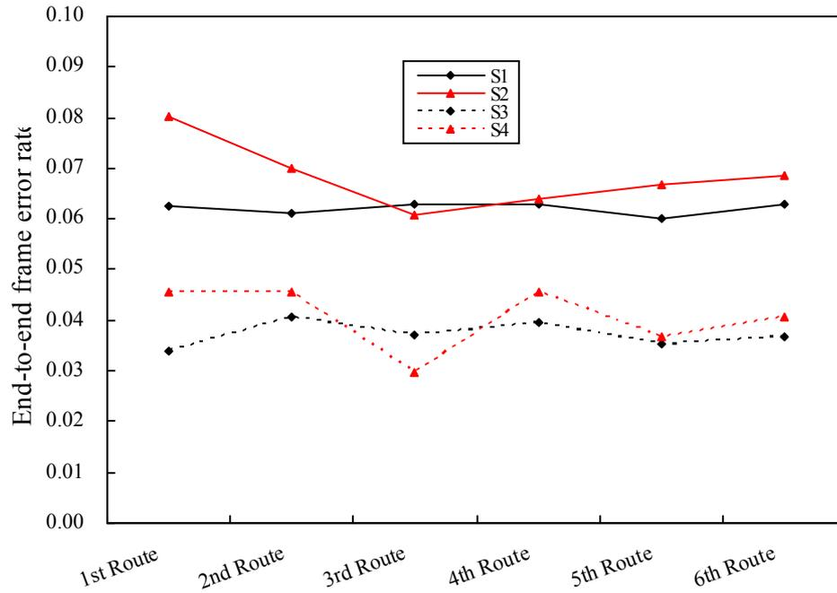
Figure 5-8: End-to-end frame error rate on each route (without ARQ).
