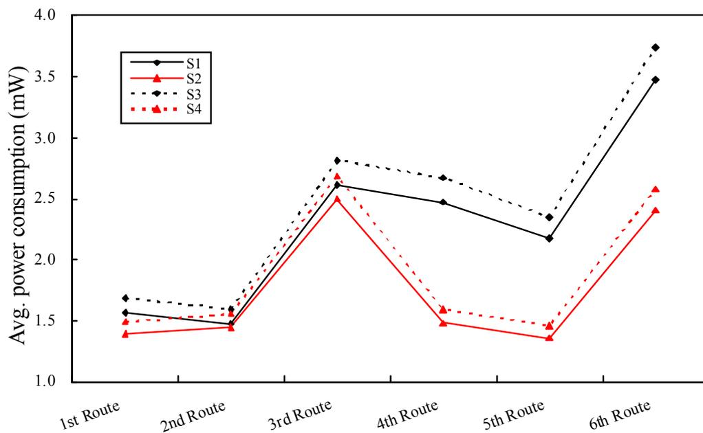
Figure 5-7: Average power consumption without using ARQ scheme.
