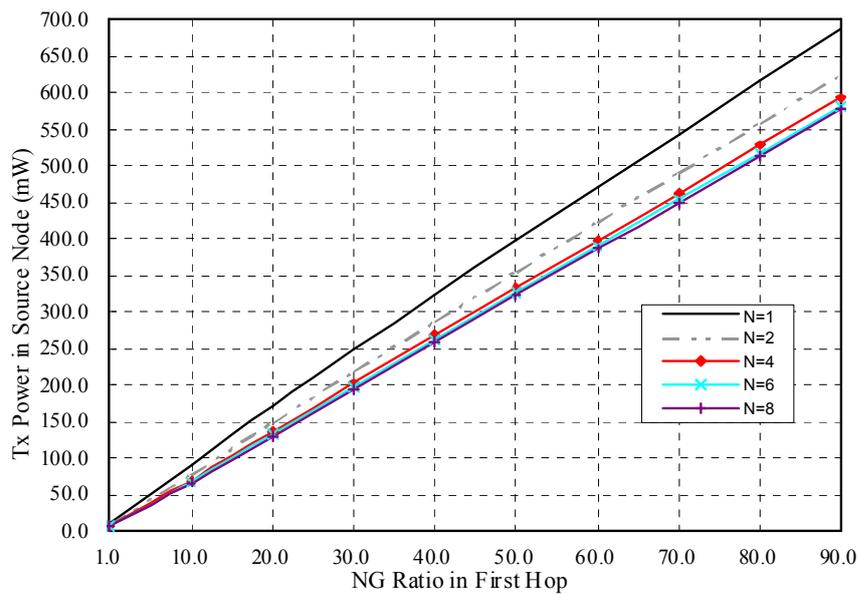
Figure 5-2: Optimal power vs.  $NG$  ratio.
