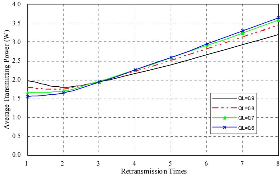
Figure 5-3: Average power consumption vs. retransmission times.
